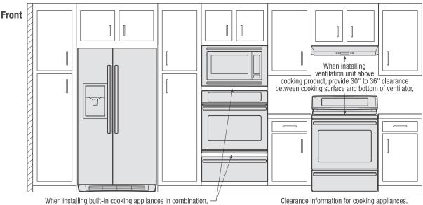
2"-high minimum visible gap between appliance faceplates required.
