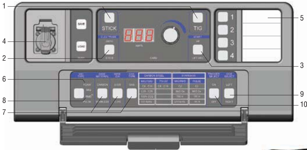
PipeWorx Power Source Control Panel with Door Open
